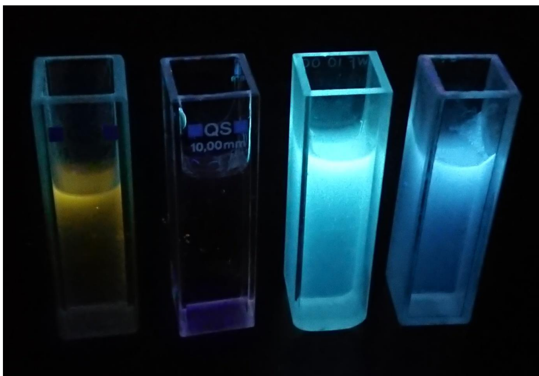
Figure S6: Fluorescence color of compound 11b in MeCN/water mixture (from left to right: 0% 50%, 80% 97% of water) The picture was taken in the dark upon irradiation with a handheld UV lamp ( \lambda_{em} = 366 nm).
