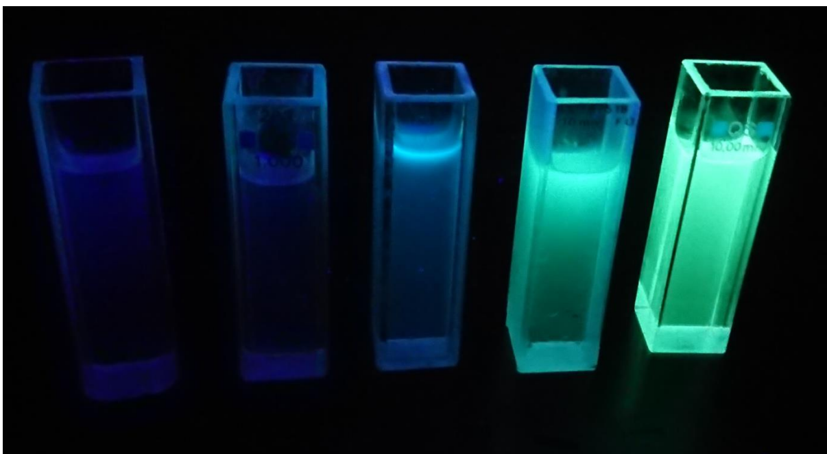
Figure S4: Fluorescence color change experienced by 11b in various solvents (from left to right: n-heptane, toluene, 1,4-dioxane, \text{CHCl}_3 , DCM) The picture was taken in the dark upon irradiation with a handheld UV lamp ( \lambda_{em} = 366 nm)
