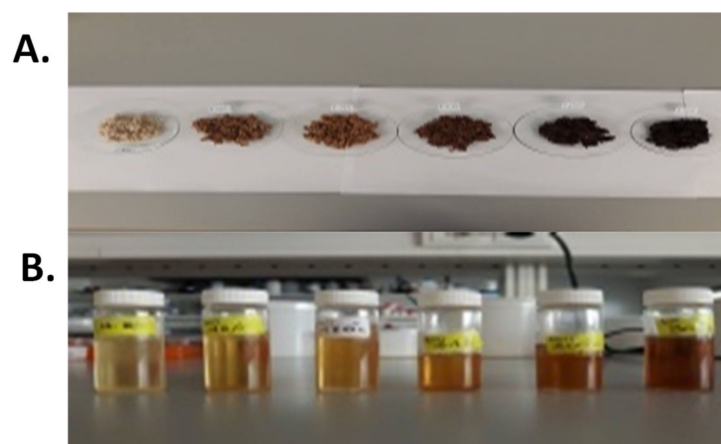
Figure 1. (A) Unroasted and roasted sesame seeds at different temperatures (top) and (B) their corresponding oils (bottom). From right to left: unroasted, roasted at 150, 180, 210, 250 and 300 °C, respectively.
