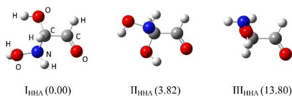
Figure 6. The optimized structures of the three most stable forms of hydroxy(hydroxyamino)acetaldehyde, HHA . The computed \Delta E_{(\text{ZPE})} energies of HHA conformers with respect to the energy of the most stable conformer, I_{\text{HHA}} , in \text{kJ mol}^{-1} are given in parentheses.
