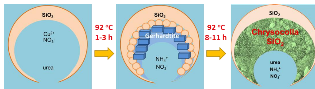
Figure 10. Simplified schematic representation for the synthesis of \text{Cu}_2\text{Si}_2\text{O}_5(\text{OH})_2/\text{SiO}_2 material.
