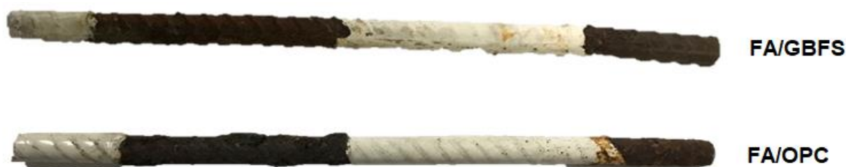
Figure 8. Rebar bars recovered after accelerated corrosion tests.
