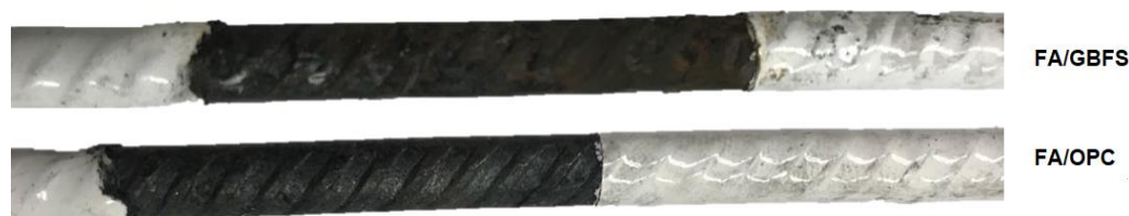
Figure 12. Photographs of reinforcing steels extracted from FA/GBFS and FA/OPC concretes, at the end of exposure to a 3.5% NaCl solution.
