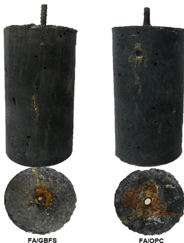
Figure 7. Photographs of the concretes after the impressed voltage test.
