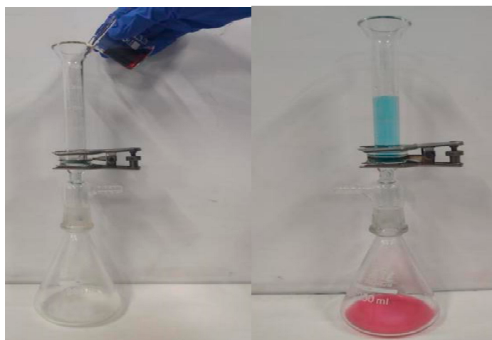
Figure S3. Oil/water separation test using the fabricated mesh.
