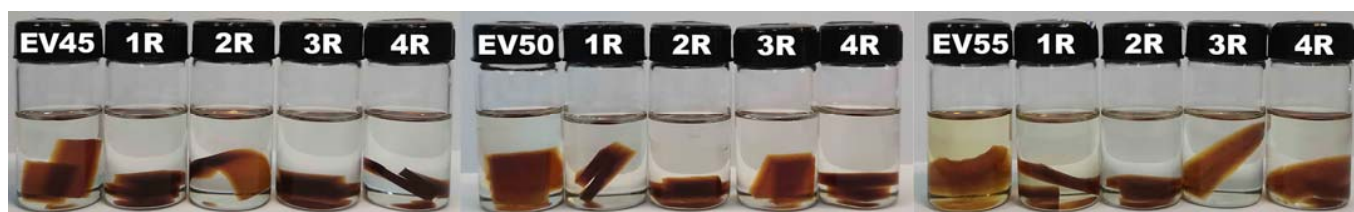
Figure 5. Solvent stability of the original and recycled epoxy vitrimers in toluene at room temperature after 48 h.
