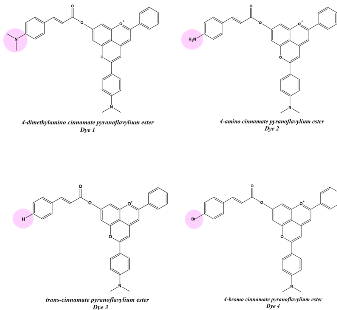
Figure 1. New dyes obtained by the esterification between cinnamic acids and a 7-hydroxyl pyranoflavylum derivative using the EDC coupling agent.
