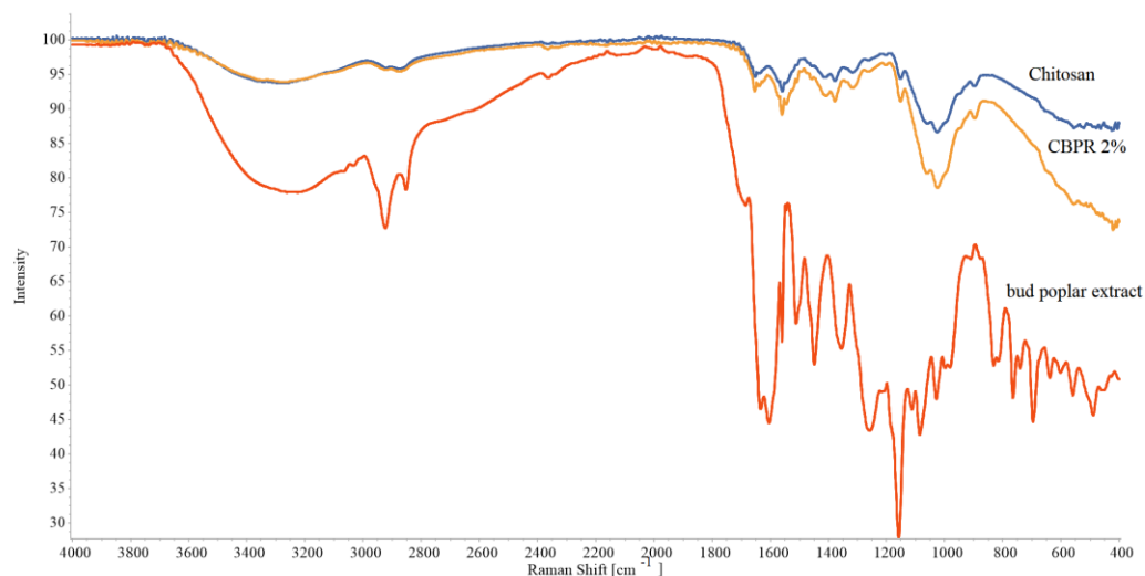
Figure 2. ATR-FT IR spectra of chitosan film, CBPR 2%, and bud poplar extract.
