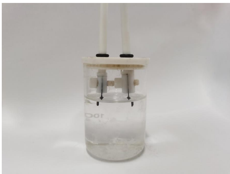
Figure S10. Photos of a two-electrode system of the Zn-Co 3 O 4 @CW-230 liquid-
