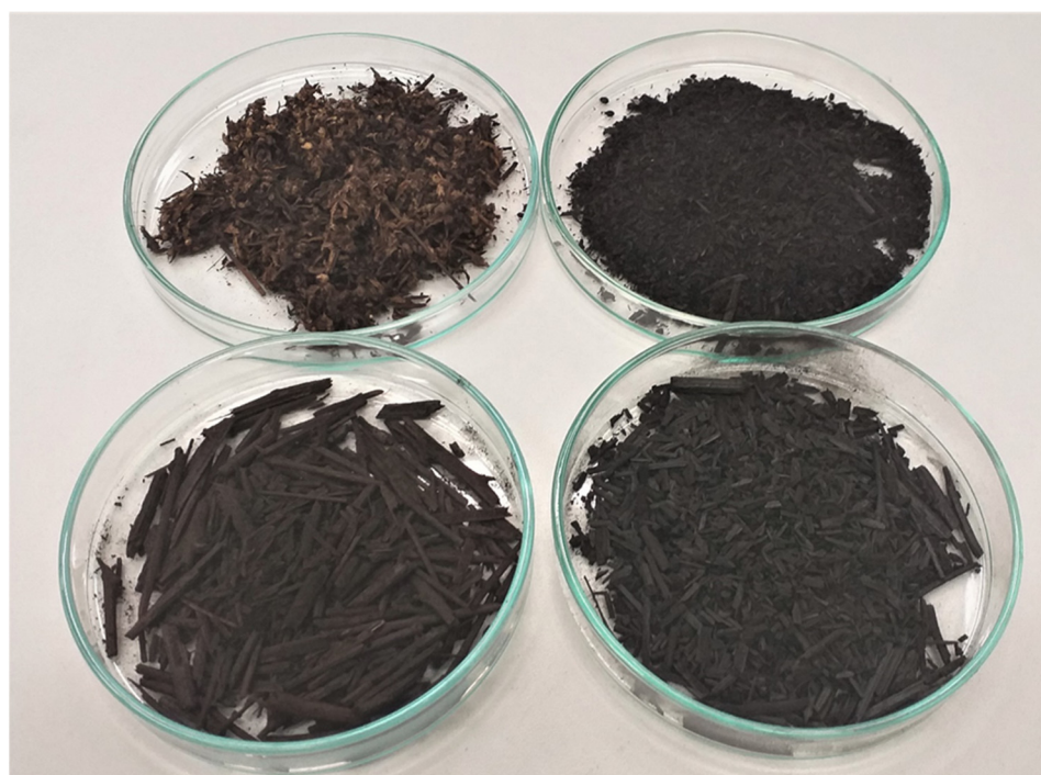
Figure 9. Pyrolysis products obtained at a temperature of 300 and 400 °C.
