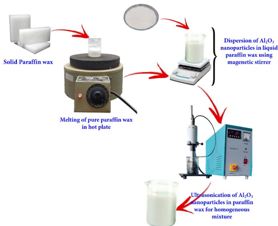
**Figure 1.** Preparation of paraffin wax with Al<sub>2</sub>O<sub>3</sub> nanoadditive.
