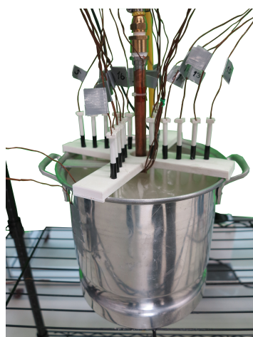
Figure 4. Cylindrical unit with thermocouple array for temperature sensing.
