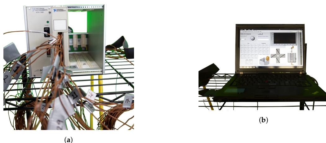
Figure 5. Data acquisition and processing system. (a) Data acquisition system. (b) Laptop for temperature data processing.
