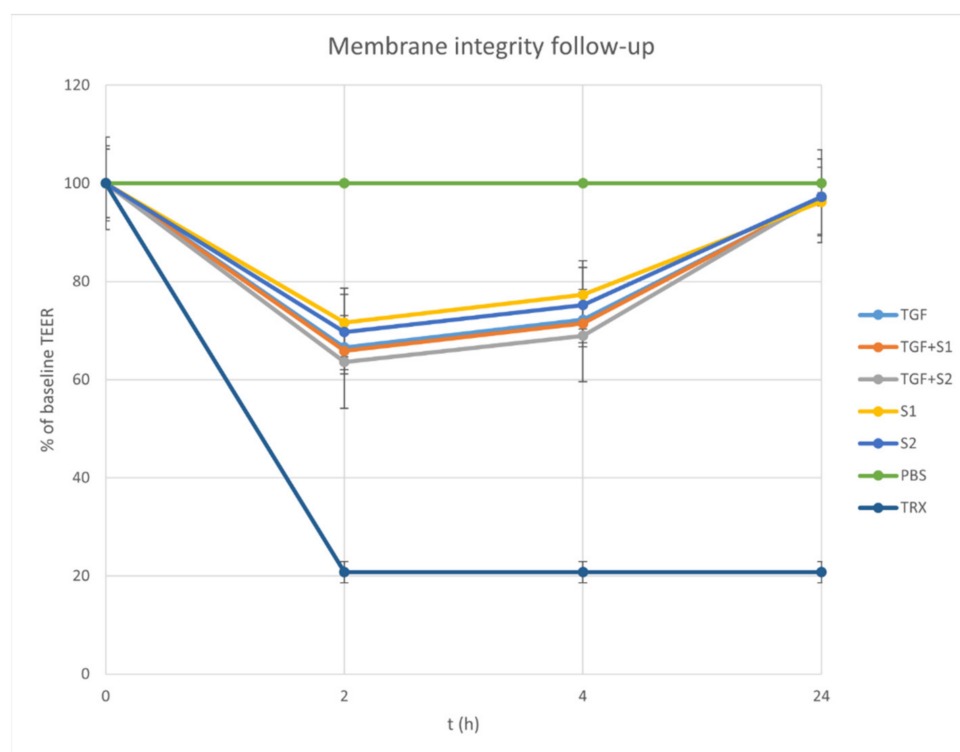
Figure 8. Trans-epithelial electrical resistance from the start of the permeability test to 24 h later. Triton-X was used as a positive control. The samples added to the inserts loosened the tight junctions of the cell layer, but in the fresh medium these were restored slowly. The TEER after 24 h was close to the baseline, which points to the survival of the cells in the fenugreek compositions. The reduction in TEER caused by Triton-X was constant until the end of the measurement, because the cells did not survive.
