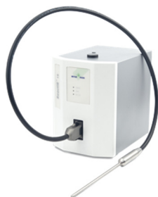
Figure S1. Mettler-Toledo ReactIR 15 equipped with diamond probe.
