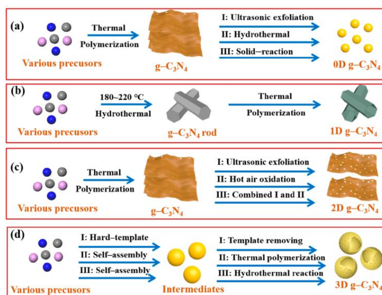
Figure 3. Schematic illustration of different techniques for the synthesis of (a) 0D g-C 3 N 4 , (b) 1D g-C 3 N 4 , (c) 2D g-C 3 N 4 , and (d) 3D g-C 3 N 4 . Reprinted with permission from Ref. [25]. Copyright 2021 American Chemical Society.
