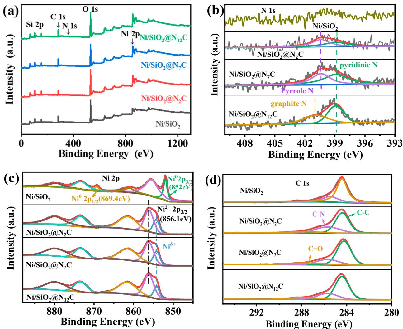
Figure 3. (a) XPS survey; (b) XPS Ni 2p spectra; (c) XPS N 1s spectra; and (d) XPS C 1s spectra of different samples.
