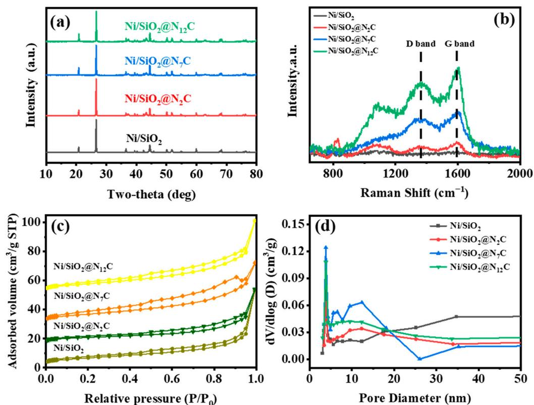
Figure 1. (a) XRD patterns; (b) Raman spectra; (c) N<sub>2</sub> adsorption–desorption isotherms; and (d) pore size distribution curves of different samples.
