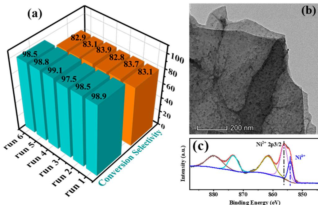
**Figure 6.** (a) recycling tests of selective hydrogenation of cinnamaldehyde over Ni/SiO<sub>2</sub>@N<sub>7</sub>C catalyst; (b) HRTEM image; and (c) XPS Ni 2p spectra of the used samples. Reaction conditions: 50  $\mu$ L CAL, 50 mg catalyst, 6 mL ethanol as solvent, 2 MPa H<sub>2</sub>, reaction temperature 100  $^{\circ}$ C, and reaction time 2 h.
