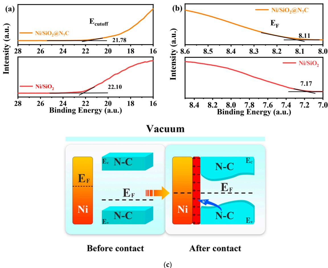
**Figure 5.** (a,b) UPS spectra of Ni/SiO<sub>2</sub> and Ni/SiO<sub>2</sub>@N<sub>7</sub>C samples (Note:  $E_{\text{cut off}}$  and  $E_F$  represent the low energy cutoff edge and the Fermi energy level, respectively); and (c) The Mott–Schottky contacting interface of metallic Ni and N-doped carbon of Ni/SiO<sub>2</sub>@N<sub>7</sub>C.
