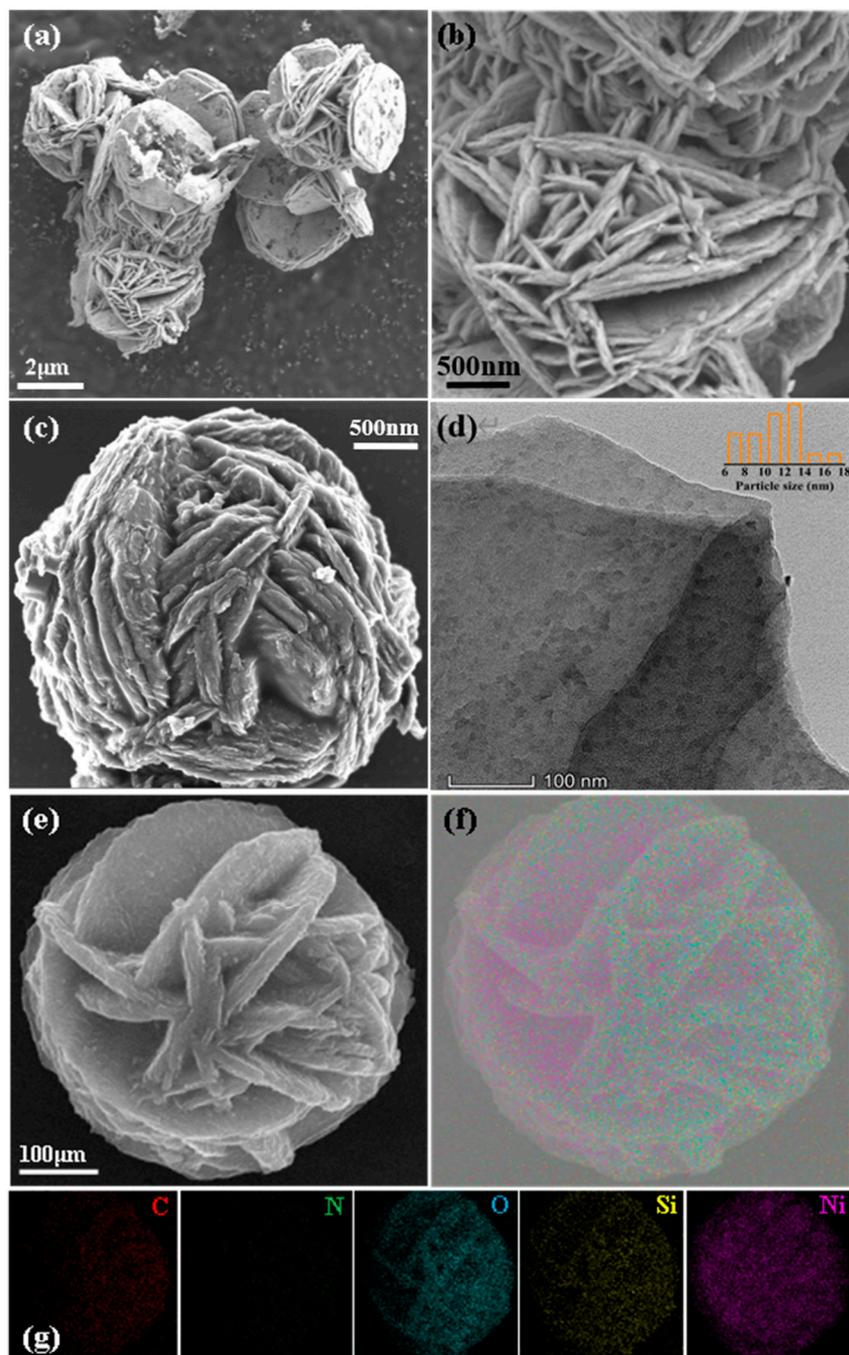
**Figure 2.** (a,b) SEM image of Ni/SiO<sub>2</sub> support; (c) SEM; (d) HRTEM; (e) STEM-HAADF; and (f,g) element mapping images of Ni/SiO<sub>2</sub>@N<sub>7</sub>C.
