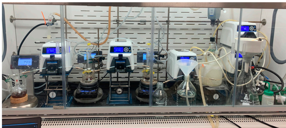
Figure S12. Fume Hood Setup for Run 3. PTFE pump heads and PTFE tube sets were purchased and implemented without the use of C-Flex tubing.
