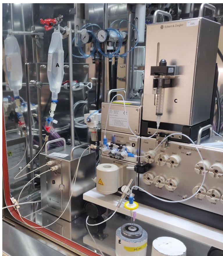
Figure 6. Synthesis setup. A: 0.1 N HCl; B: GalliaPharm ^{68}\text{Ge}/^{68}\text{Ga} -generator; C: dispensing syringe; D: Stopcock manifold; E: lead shield with product vial.
