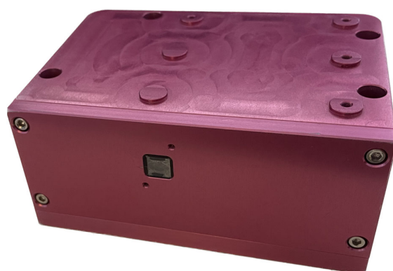
Figure 9. Experimental instrument—portable NIR spectrometer.
