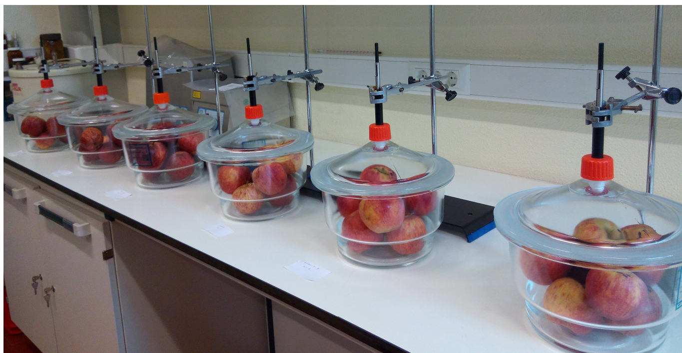
Figure 1. HS-SPME collection of volatiles from pooled samples of 7 ‘Gala’ apples (“Maçã de Al-cobaça”) per desiccator at room temperature.
