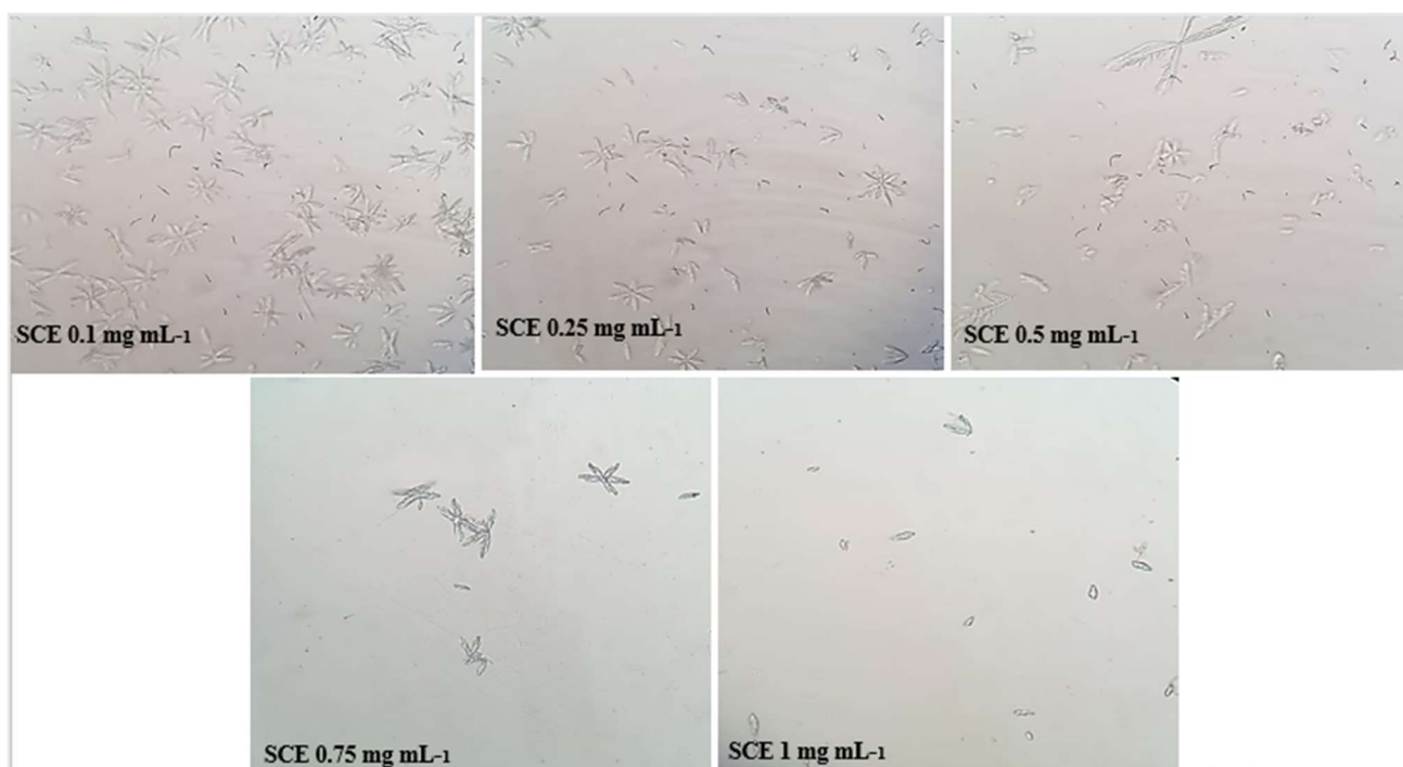
Figure 2. Microscopic observation of struvite crystals at different concentrations of ethanolic extracts of S. costus .
