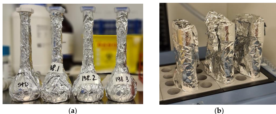
Figure 9. Preparation of oleoresin samples for the HPLC analysis. (a) 100-mL amber glass flasks wrapped with aluminium foil with stock solutions. (b) Pyrex tubes wrapped with aluminium foil during hydrolysis.
