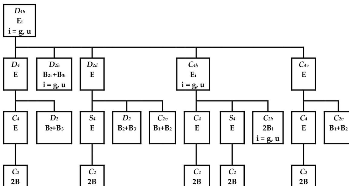
**Figure 5.** Possible symmetry descent paths of  $D_{4h}$  structures in double degenerate electron states [9]. The top and bottom lines of individual rectangles denote symmetry groups and the corresponding irreducible representations, respectively.
