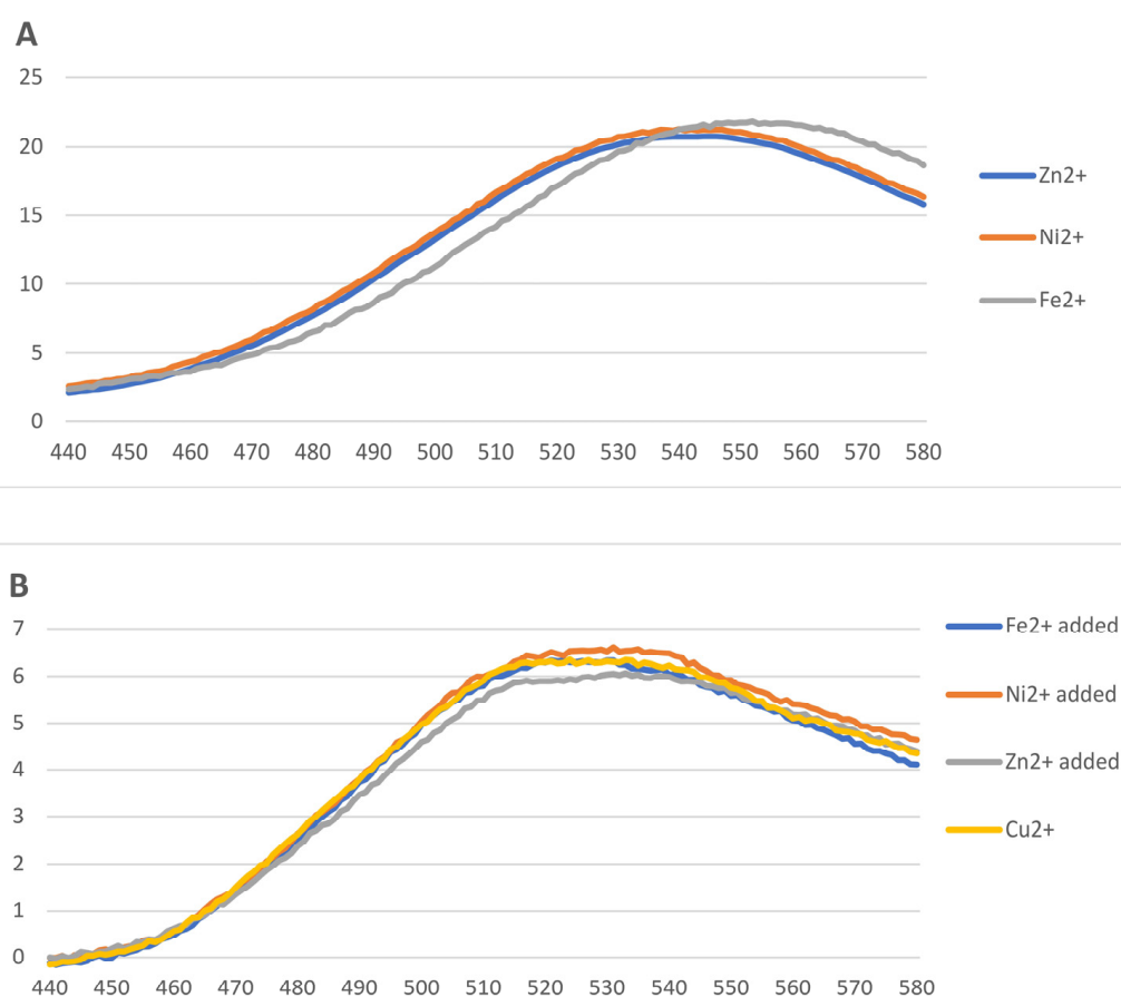
Figure 7. Response of indicator 8 (0.1 M MES buffer, pH 6.0, 0.005 g/L) to other metal ions in presence of \text{Cu}^{2+} . (A) response to \text{Zn}^{2+} , \text{Ni}^{2+} , and \text{Fe}^{2+} alone (10 \mu\text{M} each). (B) response of competing metal ions against \text{Cu}^{2+} , showing response to \text{Cu}^{2+} and response from addition of \text{Fe}^{2+} , \text{Ni}^{2+} , or \text{Zn}^{2+} , each 10 \mu\text{M} . \lambda_{\text{ex}} = 330 \text{ nm} ; excitation slit width = 10; and emission width = 10.
