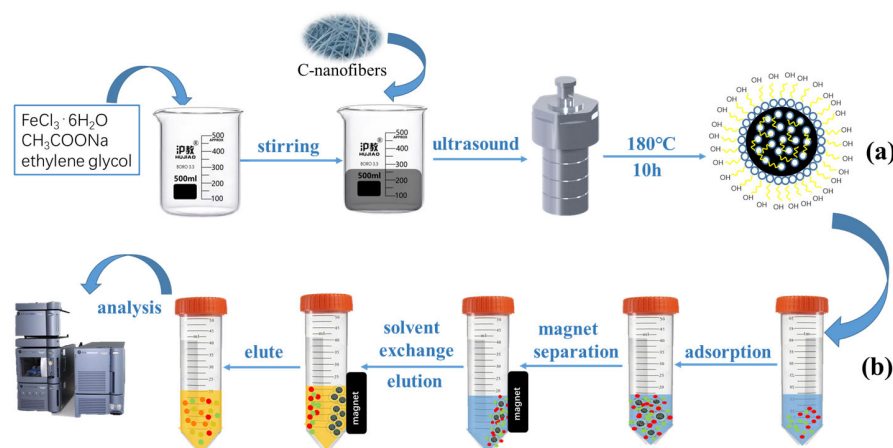
Figure 5. A schematic diagram for the preparation of the \text{Fe}_3\text{O}_4@\text{C-NF} nanocomposites (a) and their application for TCs extraction (b).
