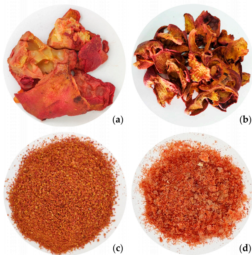
Figure 4. (a) Fresh pomegranate waste; (b) Dried pomegranate peel; (c) Pomegranate peel powder; (d) Dried pectin obtained at optimal extraction conditions.
