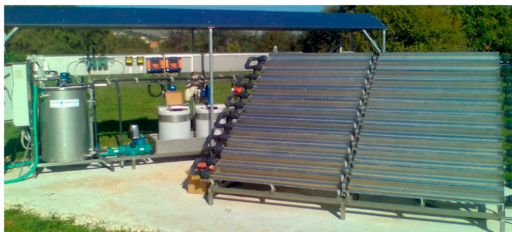
Figure 5. Photograph of CPC photocatalytic pilot plant established in the secondary effluent of WWTP facility of University Hospital, Ioannina city.
