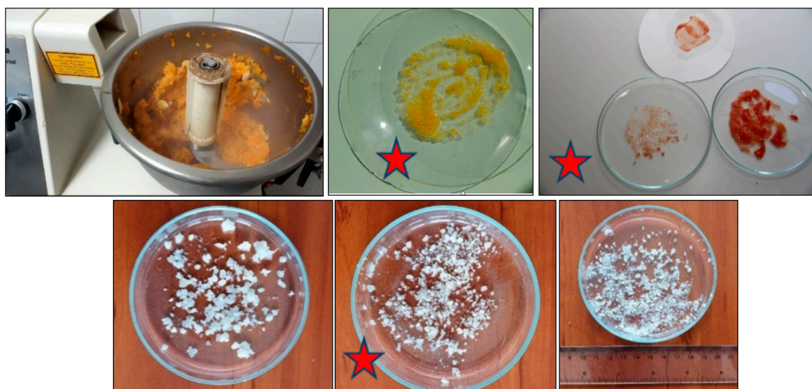
Figure 5. Top row left Blending winter squash; top center and right: tomato homogenates on filter paper and Petri dish; second row: cabbage leaves homogenized to different particle sizes. The star marks the acceptable particle size distribution.
