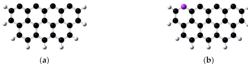
Figure 2. The optimized structure of typical models. (a) The carbonaceous surface, abbreviated as char. (b) The carbonaceous surface decorated with one pyridine group, abbreviated as charN.
