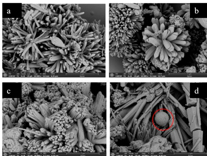
Figure 12. SEM images of (a) \text{Fe}_1\text{Co}_3\text{-MOF-74} , (b) \text{Fe}_1\text{Co}_2\text{-MOF-74} , (c) \text{Fe}_2\text{Co}_1\text{-MOF-74} , and (d) \text{Fe}_3\text{Co}_1\text{-MOF-74} . Adapted with permission from Ref. [81], 2023, Elsevier.
