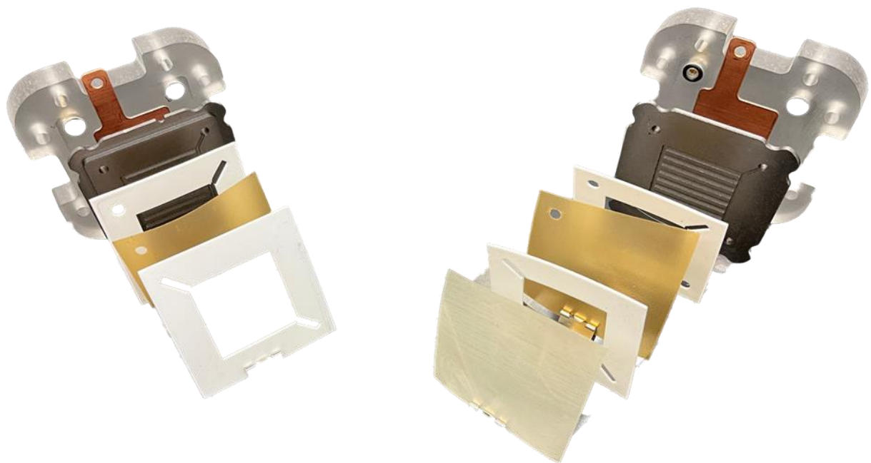
Figure. S3. Photo of the RFD cell structure.
