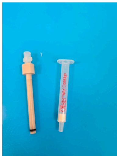
Figure 1. WAX 1cc cartridge (right) and PEEK liner with the Luer adapter (left).
