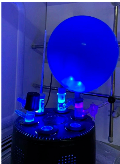
Figure S1. The photocatalytic reactor.
