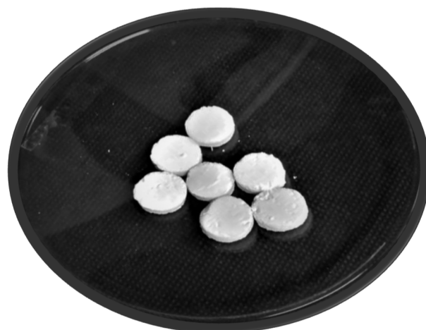
Figure 11. Shaping the sample before immersion in SBF.
