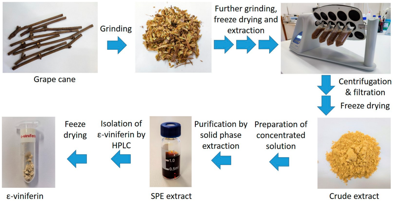
Figure 2. Key steps of grapevine cane processing to obtain crude extract and pure \epsilon -viniferin.
