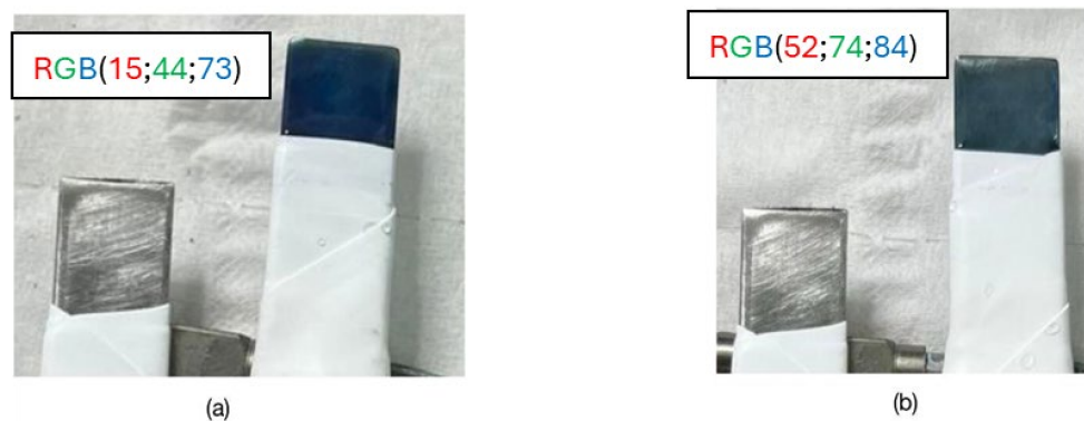
Figure 3. (a) Freshly electrogenerated PMB on SS316 in basic medium, free of \text{Cl}^- anions and with \text{C}_2\text{O}_4^{2-} ; (b) PMB on SS316 after characterization in 0.5 M \text{KNO}_3 solution. RGB coordinates of each blue electrode are marked.
