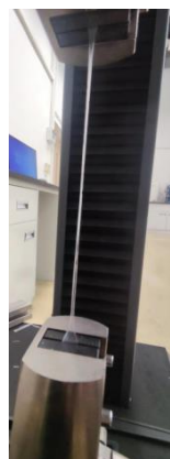
Figure S6. Deformation of TPU-20% PPG -25%HS film during tensile process.
