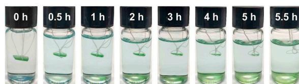
**Figure 14.** Chemical degradability of the HMDO-based thermosetting plastic. Reproduced with permission from ref. [127]. Copyright 2019 The Royal Society of Chemistry.
