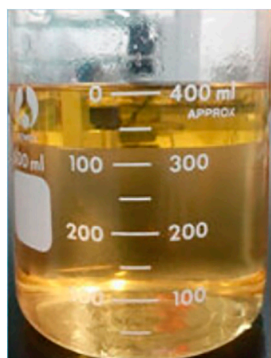
Figure 7. Phase transition phenomena of DMBA + DEEA mixed amine solvent [92].
