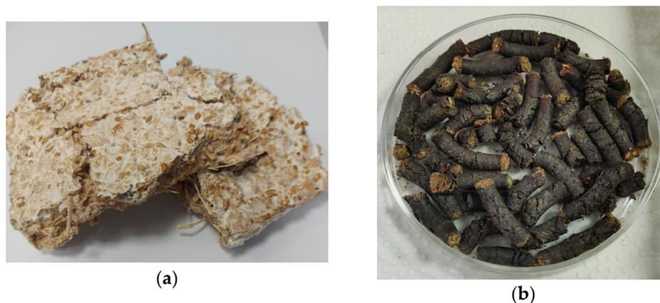
**Figure 5.** (a) Mycelium-based packaging material after compression test and (b) Coffee waste and pine wood pellets.
