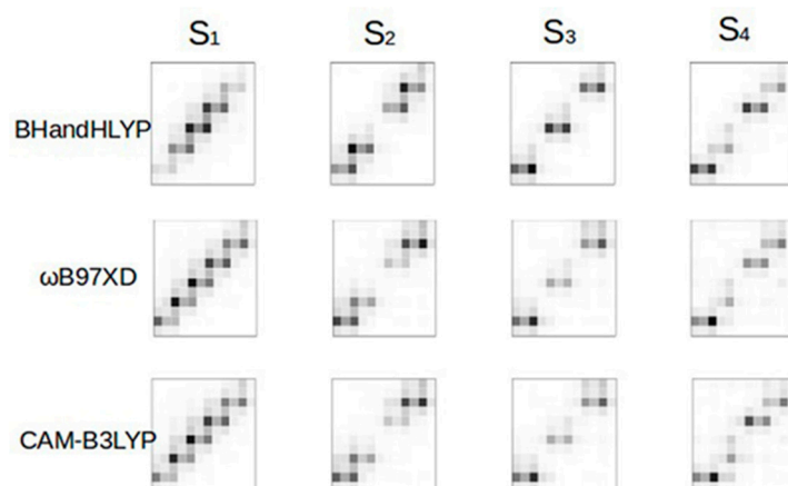
Figure S2: The transition density analysis of S 1 -S 4 for hexamer in the PC geometry at the BHandHLYP/def2-SVP, ωB97XD/6-31G* and CAM-B3LYP/6-31G* levels
