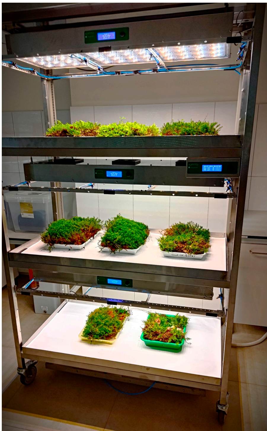
Figure S8. Moss cultivation in phytotron rack on three types of substrate: control, cement composite and MWCNT-modified cement composite
