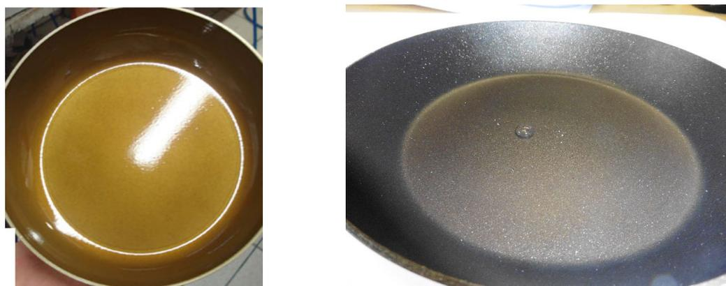
**Figure 14.** Frying pan metal base with the polyphenolic-TEP binder applied to it (**left**) and finished pan with Teflon applied on the binder according to a proprietary process (**right**) [33].
