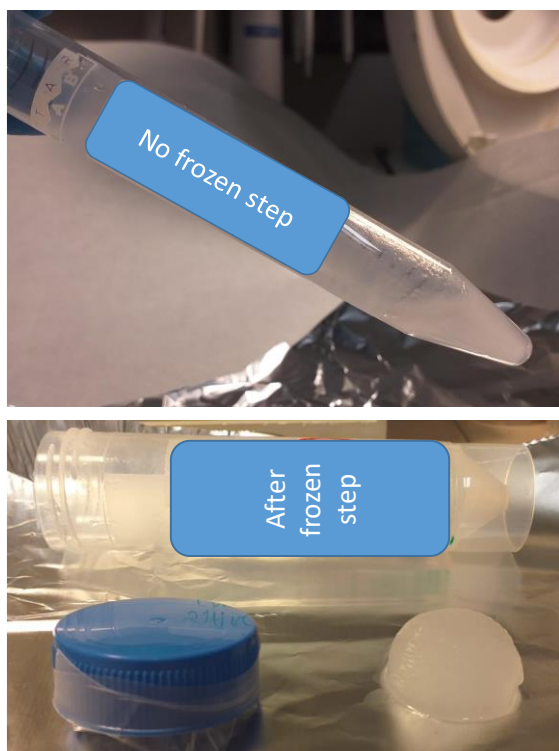
Figure S3. Macroscopical pictures of the produced materials depending on whether or not a frozen step was applied.
