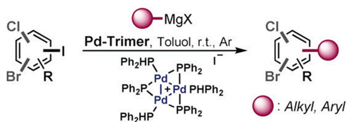
Figure 29. C–I-selective cross-coupling catalyzed by a C_3 symmetric cationic palladium trimer. Adapted with permission from ref. [150] Copyright © 2024, Wiley-VCH Verlag GmbH & Co. KGaA, Weinheim, Germany.
