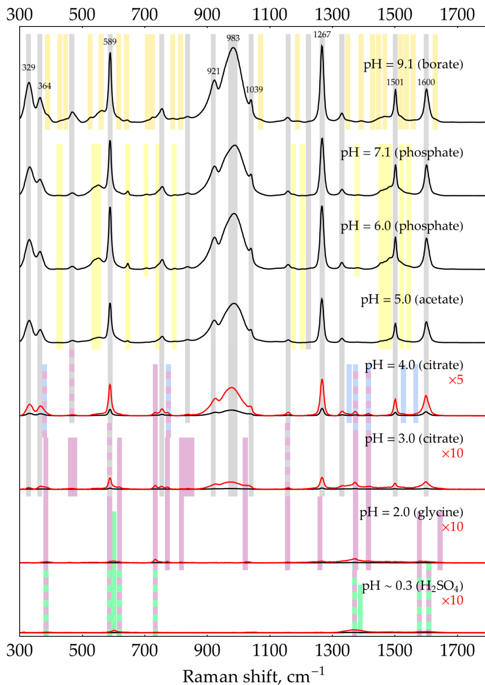
Figure A15. SERS spectra (135 mW, 785 nm, 15 s total accumulation time) of 1 mM oPD with AgNPs in 5 mM NaCl at different pHs. The polynomial baseline was subtracted from each spectrum. Black lines represent original spectra; red lines represent multiplied ones for visual clarity. Shading: grey—neutral oPD, orange and yellow—oxidation products of oPD, blue—DAP, purple—DAPH + , green—DAPH 2 2+ .
