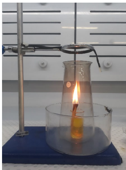
Figure 10. Illustration of the carbon soot deposition process on untreated CF tow. This modification process offers a simplified and efficient alternative to intricate methods for incorporating CNOs onto carbon fibers, addressing the challenges associated with complex and chemical-intensive techniques commonly used in the field. The presented approach allows for uniform CNO coverage on the CF surface, paving the way for enhanced interfacial interactions in CFRTPs.
