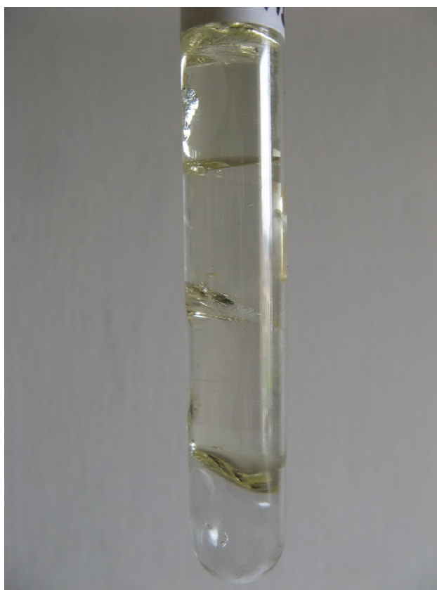
Figure 13. Photograph of a test tube containing the hyper-branched polymer synthesized with HDI and PEG350M at a molar ratio of 1:1. The three V-shaped gaps/cracks observed in the polymer are the result of the significant contraction of the material, as it solidified into a soft rubbery state within the incubation period at room temperature.
