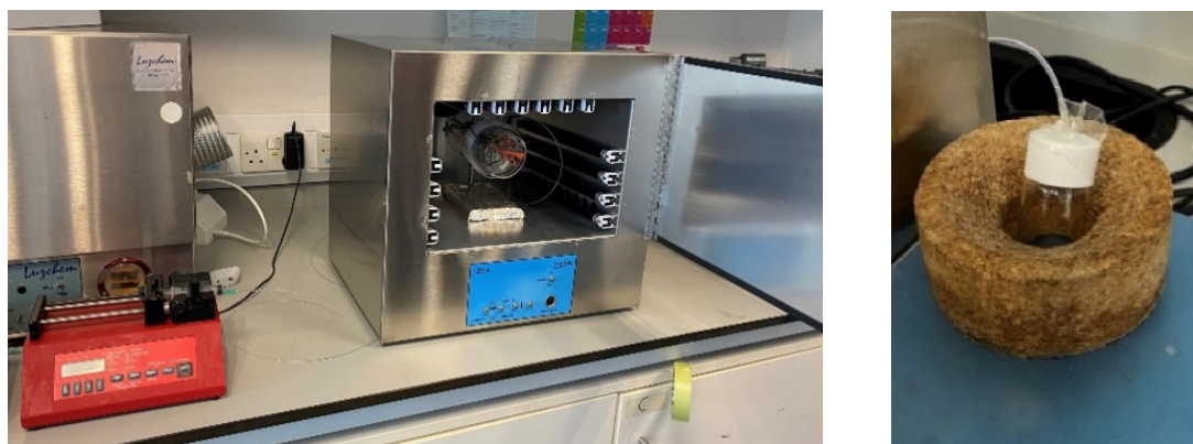
Figure S2. UV flow reactor set-up. Syringe pump with a 10 mL syringe containing the reaction mixture was connected to FEP tubing (inner diameter 0.8 mm) coiled around a glass insert placed inside a Luzchem photoreactor, LZC-EDU (110 V/60 Hz) containing 14 UVA lamps centred at 354 nm (left). The terminus of the tubing was inserted into a glass vial outside the UV reactor for sample collection (right).
